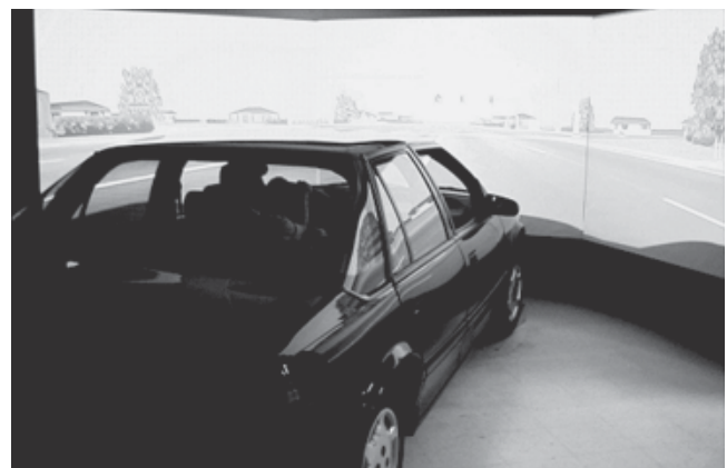
FIGURE 1 University of Massachusetts at Amherst driving simulator (Saturn sedan and three screens).
